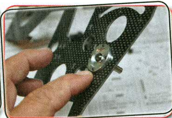
Frames are made from carbon fibre
