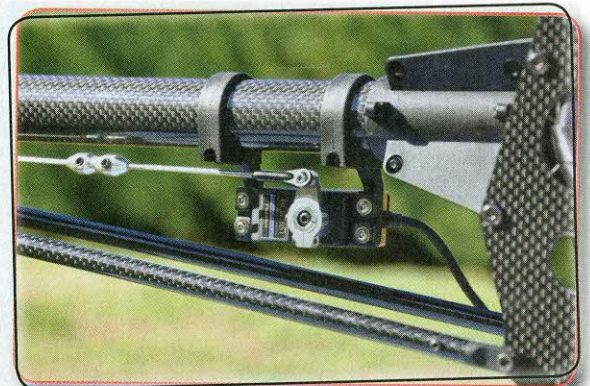
Tail servo is neatly wired up
