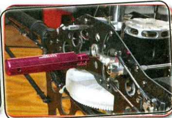
Mainshaft locked in place
