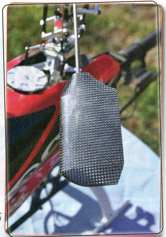
Standard carbon fibre fly-bar paddles are supplied
