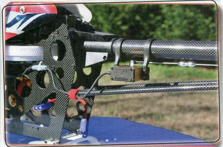
Tail servo is neatly wired up
