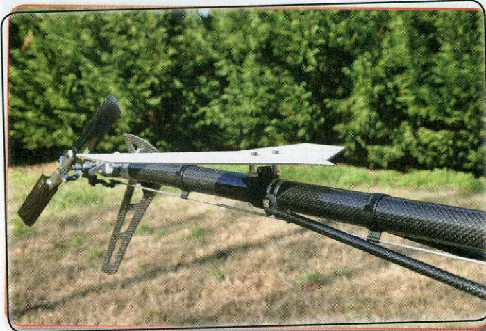
Horizontal tail fin fitted especially for F3C contest flying
