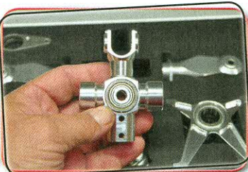
Rotor-head uses a pinned pivot point
